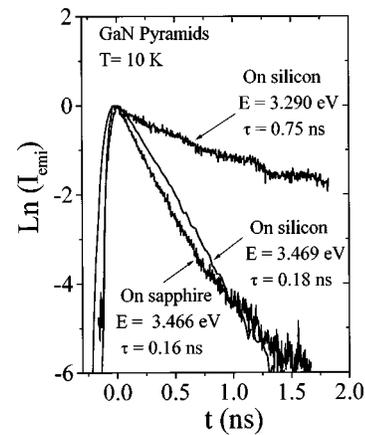
FIG. 3. PL temporal responses measured at 10 K and at emission energies  $E=3.294$  and  $3.469$  eV for the GaN pyramids overgrown on the GaN/AlN/silicon substrate, and at  $E=3.466$  eV for the GaN pyramids overgrown on the GaN/AlN/sapphire substrate.
