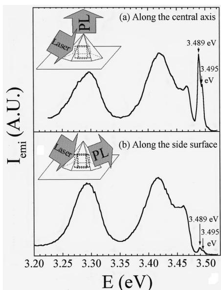
FIG. 4. Low-temperature PL spectra of the GaN pyramid overgrown on the GaN/AlN/sapphire substrate collected along (a) the central axis and (b) one of the six surfaces of the pyramid.
